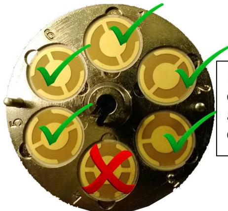
Ensure the gap in the crystal connector is not adjacent to the connector pin position
