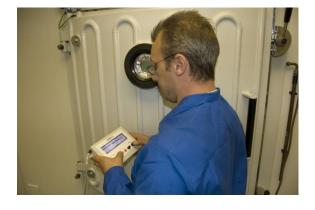
The programmable Genius deposition controller regulates all aspects of the electron beam deposition process. As well as controlling the high voltage and regulating the filament supply, the Genius also handles the magnet current supply to the coils of the electron beam evaporator.
