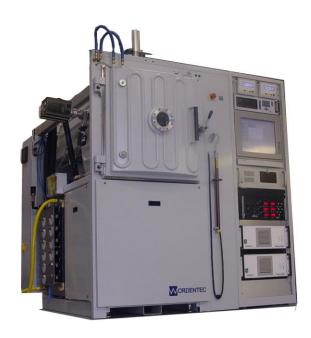
Upgraded Wordentec BAK600 System. Ferrotec Carrera high voltage supplies are fitted in the single control rack.
